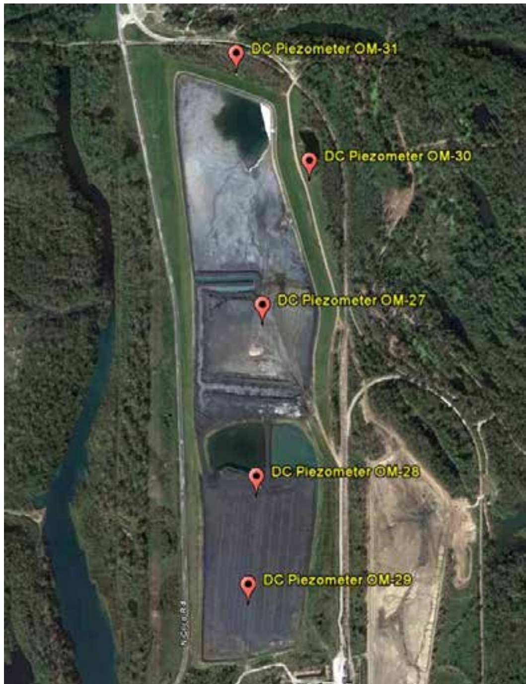
Figure C.1. Piezometer locations for Ash Pond No. 1 and Ash Pond No. 2.
